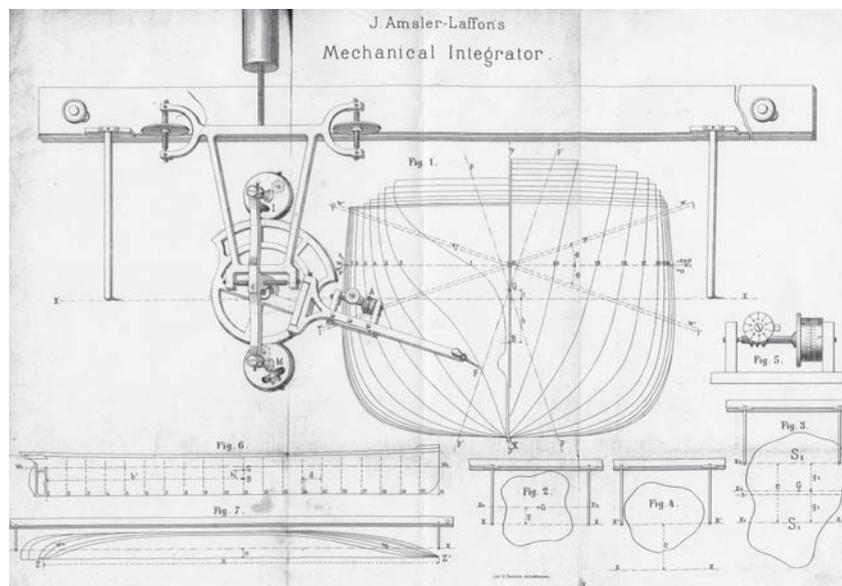
This training drawing illustrates the measurement of stiffness, displacement, and stability of a complex ship's hull design. A few measurements replaced weeks of hand calculations.
