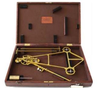
The Integrator quickly calculates the bending properties of any railroad rail design placed under it. The user need only trace the outline. This complex mechanism calculates static and inertial moments as a drawing is traced.
