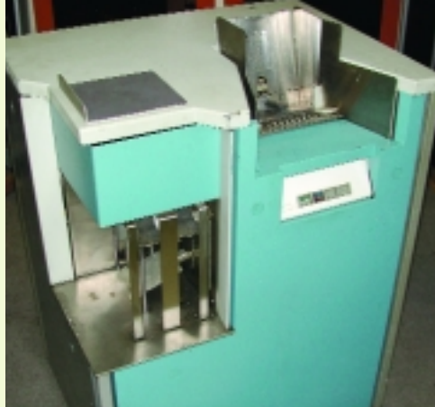
The card reader, the primary input device for programming the Sigma 5
