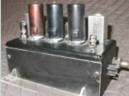
English Electric, DEUCE Mercury Delay Line Amplifier Circuit (1955), XD 4.75, Gift of Murray Allen.
