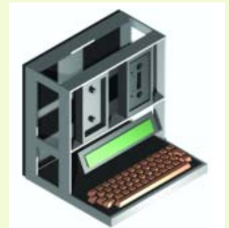
The MCM/70 desktop bare-bones system. 3D model created by André Arpin.
