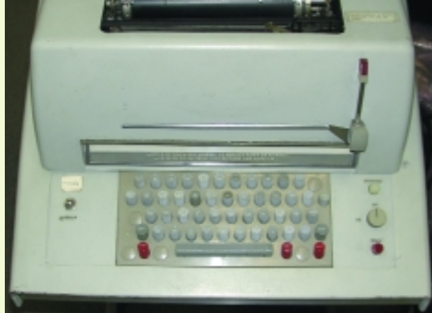
Console teletype. Through the mid-1970s, most mainframe computer systems used hardcopy terminal as consoles to aid in resource accounting, operator tasks, and general system debugging. The Sigma 5 was unusual in that it employed a TTY utilizing EBCDIC rather than the more common ASCII character encoding.
