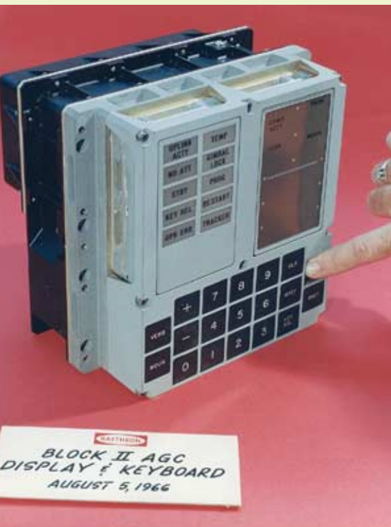
The interface with the astronauts was the DSKY (for display keyboard). It used digital displays and communicated with the astronauts using verb and noun patterns and two-digit operation and operand codes. A set of status and caution lights is shown in the top left corner.
