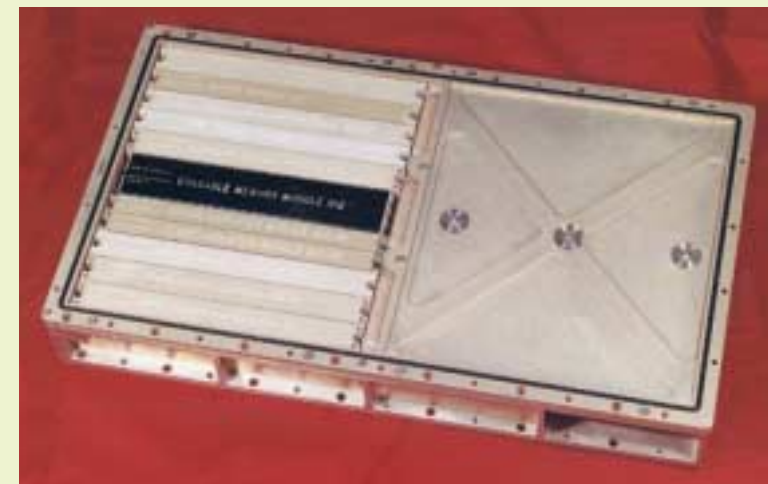
The Apollo Guidance Computer was responsible for the guidance, navigation, and control computations in the Apollo space capsule. The AGC was the first computer to use integrated circuit logic and occupied less than one cubic foot of the spacecraft. It stored data in 15-bit words plus a parity bit and had a memory cycle time of 11.7 microseconds, utilizing 2,000 words of erasable core memory and 36,000 words of read-only memory. The frame is made of magnesium for lightness and designed to hermetically seal the components.
