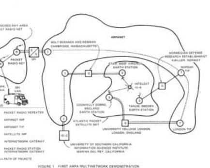
(top) Diagram of the first two-network internet transmission on August 27, 1976. (Original illustration from an SRI technical report "Progress Report on Packet Radio Experimental Network" published in September 1977.)
