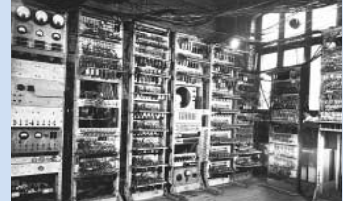
While working for Williams, Kilburn and Tootill built the Baby to demonstrate the viability of CRTs for storage (memory). It worked successfully for the first time on June 21, 1948, becoming the world's first functioning stored program electronic computer.
