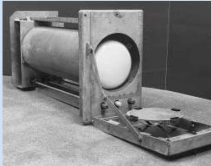
The Williams Tube cathode ray tube memory system pioneered by Kilburn and Williams was used around the world by computer systems as an alternative to mercury delay line stores until the mid 1950s, when both were supplanted by core memory.
